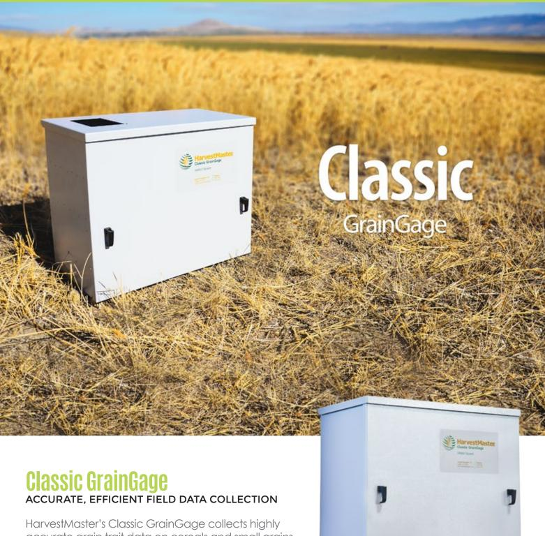
HarvestMaster's Classic GrainGage collects highly accurate grain trait data on cereals and small grains, even for samples as small as 900 grams. Multiple samples are processed from a plot to provide reliable measurements for moisture, test weight, and plot weight. With the Classic GrainGage, you can record
